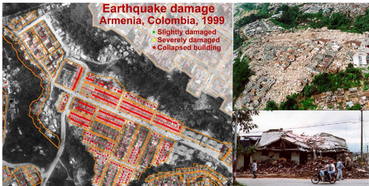
Figure 3: Left: Orthophoto made with aerial photographs of 1999, taken few days after the earthquake, overlain by the city blocks and point map indicating damaged buildings of Barrio Brasilia in Armenia. Upper right: Oblique aerial photo of the same area. Lower right: Field-photo showing example of roof collapse.
