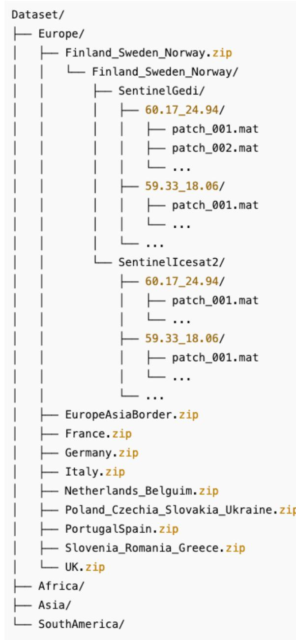
Each MATLAB **\*.mat** file represents a 256×256-pixel co-registered Sentinel-1 and LiDAR patch, containing the following variables:
