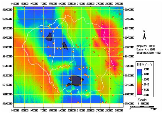
Figure 1-2: SRTM-DEM, catchment boundaries, lakes and distribution of rain gauges.
