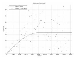
Figure 5-12: Cross-variogram model of wet-wet probability of daily rainfall and elevation.
