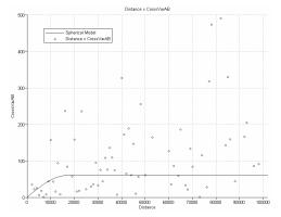
Figure 5-6: Cross-variogram model of standard deviation of daily rainfall and elevation.
