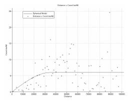
Figure 5-15: Cross-variogram model of wet-dry probability of daily rainfall and elevation.
