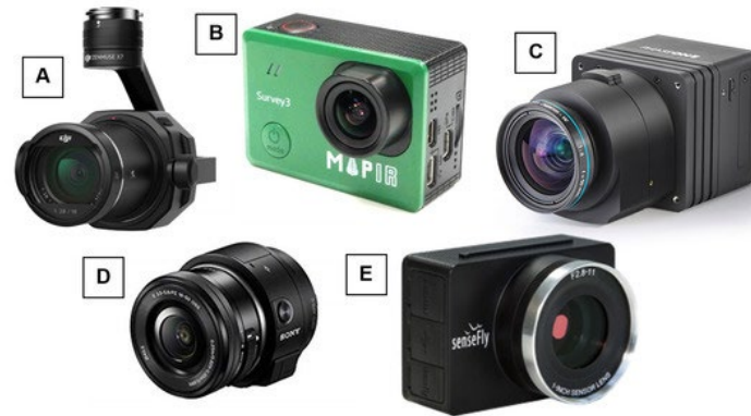
(A) DJI Zenmuse X7; (B) MAPIR Survey3 (also available in multispectral option); (C) PhaseOne iXU-RS 1000; (D) Sony ILCE-QX1; (E) senseFly S.O.D.A
