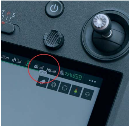
Figure 3.10 - signal strength indicator on a UA ground station.
