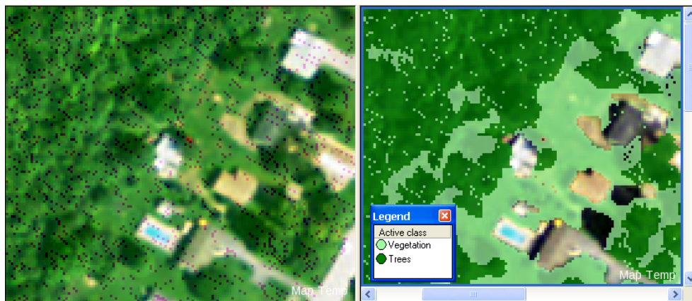
Figure 47: Left: Optical layers and Number of Returns not interpolated in mixed view; Right: Classification Result (Map Temp).
