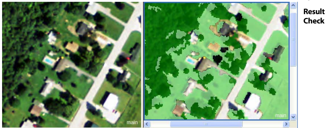
Figure 46: Left: Optical layers; Right: Classification Result using interpolated image layer 'Number of Returns Interpolated' (mainMap).
