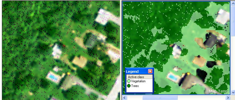
Figure 23: Left: Optical layers and Number of Returns in mixed view; Right: Classification Result.
