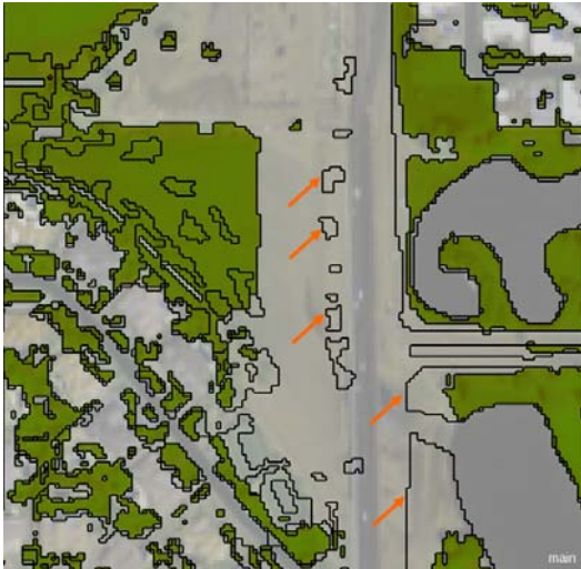
Figure 38: The outlines of the underlying Level are now also cut in the upper Level.
