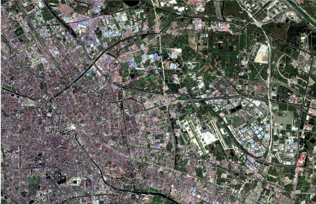
You should now see two more menus in the menu bar: **Segmentation** and **Edge Detection**. You should first go into edge detection and press the perform button. This will open a new dialog for the two parameters required for a canny based edge detector. Those are two threshold values. Set the **lower threshold** to 0.1 and the **upper threshold** to 0.2 and explore the result. These parameters are used for a gap-filling procedure during edge detection.
