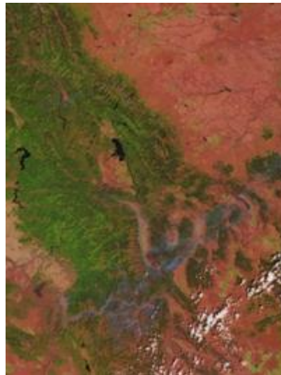
Figure 4-8: RGB image of forest fires. The image was obtained from ATSR-2's nadir view, during a day-time pass of the northwest American states of Idaho and Montana. In this representation there is a clear distinction between the cloud (white) and the smoke from the fires (blue), whilst forested areas appear green.
