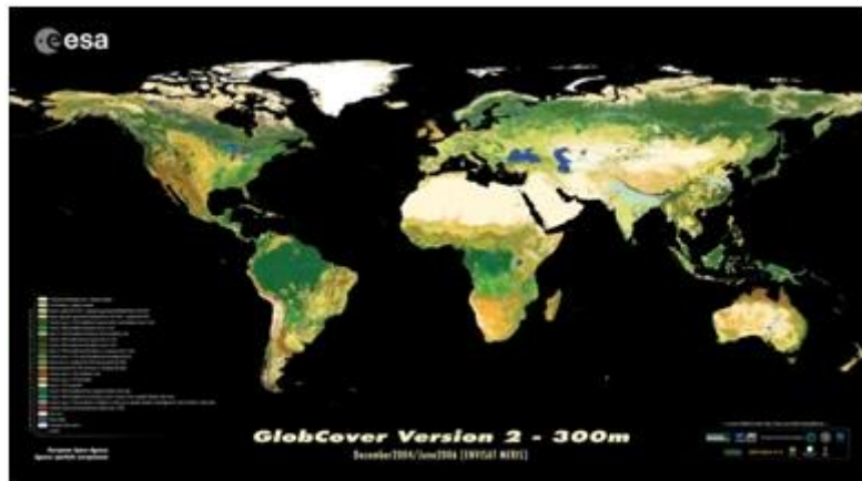
Figure 3-8: At 300 m resolution, GLOBCOVER Land Cover v2 provides a revealing portrait of global land use. To build this map, a colour representing one of 22 different land classifications is associated with each pixel. The associated land classification is define according to the predominant type of vegetation found at that location (image courtesy of ESA GLOBCOVER project).
