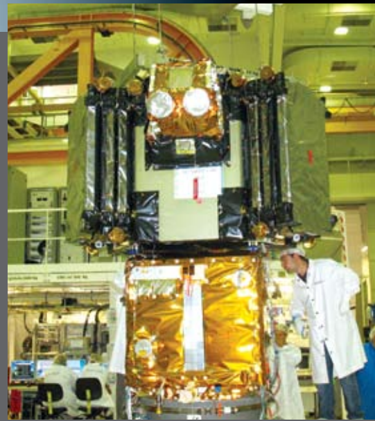
The SMOS payload and Proteus platform in the cleanroom at Thales Alenia Space in Cannes, France
