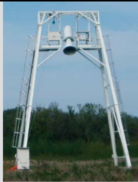
An L-band radiometer being operated at a site close to Toulouse, France. The measurements, taken over several months, were used to estimate how the vegetation at different stages of growth in different soil moisture conditions influences microwave emissions.
