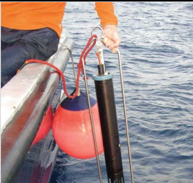
Taking calibration measurements of sea-surface salinity and temperature in the Mediterranean Sea. Simultaneous measurements were taken from a campaign aircraft flying overhead.
