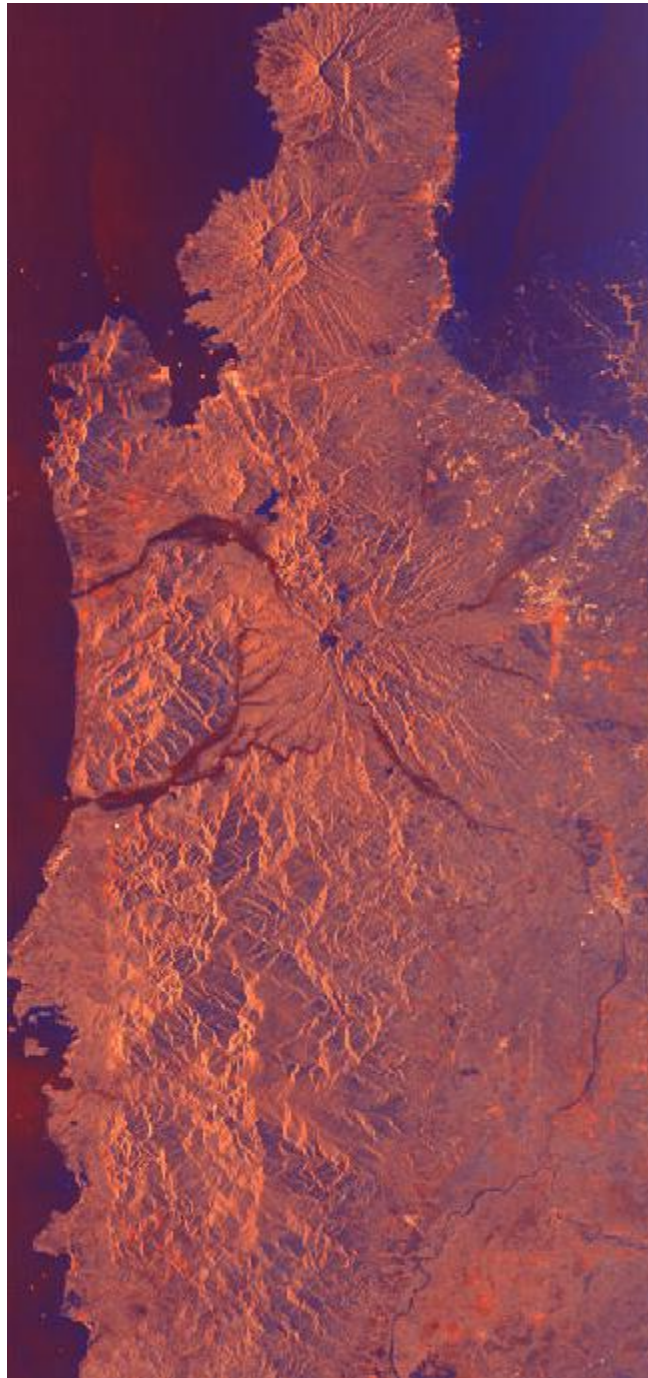
Figure 6-6 3 Channel (RGB) Composite Dual Polarisation VV/VH Quick-look Image
