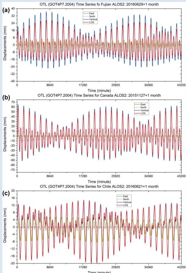
Figure 3. Time series of OTL N/E/U/LOS displacement with 30 days estimated from GOT4.7 model. The starting time is identical with the observation time of ALOS-2 PALSAR-2 master image.
