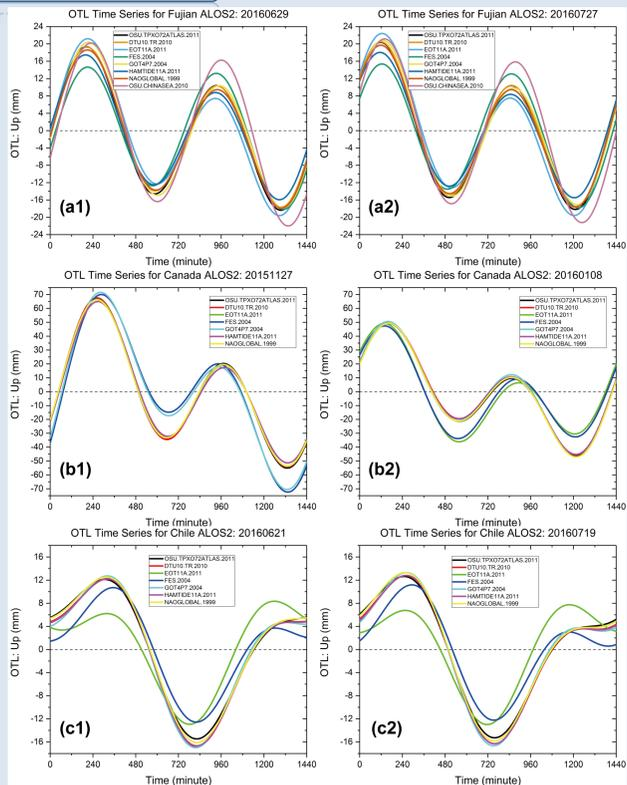
Figure 2. Time series plot of OTL vertical displacement with 24 hours estimated from multiple OTLs. The starting time is identical with the observation time of ALOS-2 PALSAR-2 master image.
