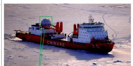
shipborne satellite remote sensing data reception system on Xuelong vessel
