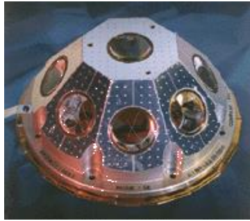
Figure 7.37. ERS-1 LRR, which is identical to the Envisat model. (Credits ESA)
