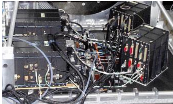
Figure 7.64. . Poseidon-2 being integrated on Jason-1. Poseidon-3 on Jason-2 is similar. (Credits CNES/Alcatel )
