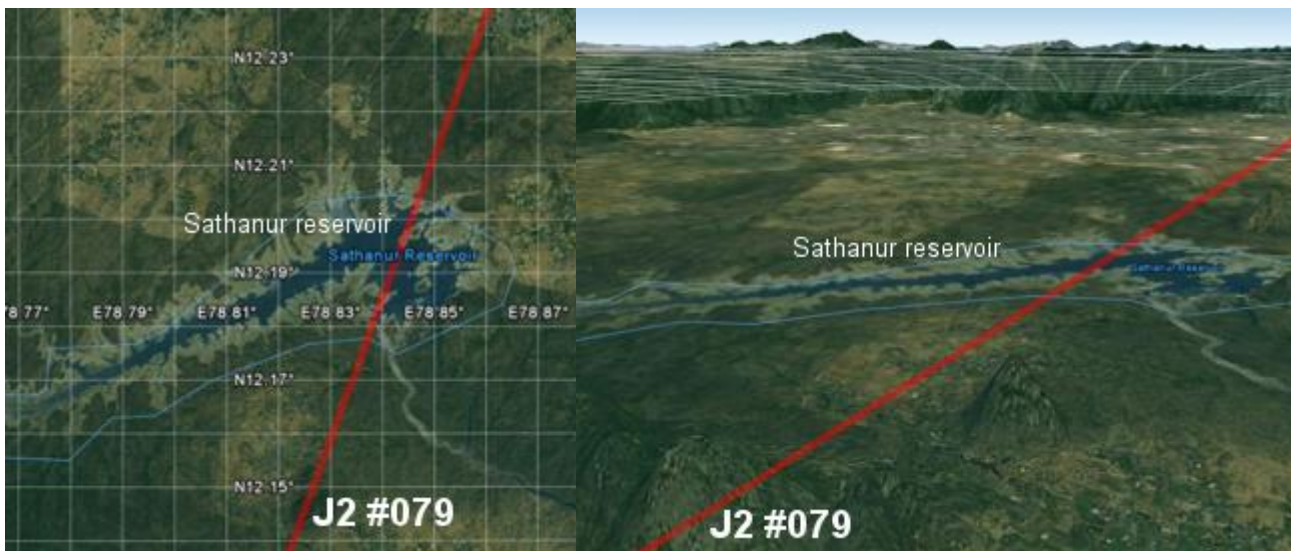
Figure 6.114. Jason-2 pass 079 overlaid on Google Earth in the vicinity of Sathanur Reservoir, India. Different views on Google Earth give important details on topography.
