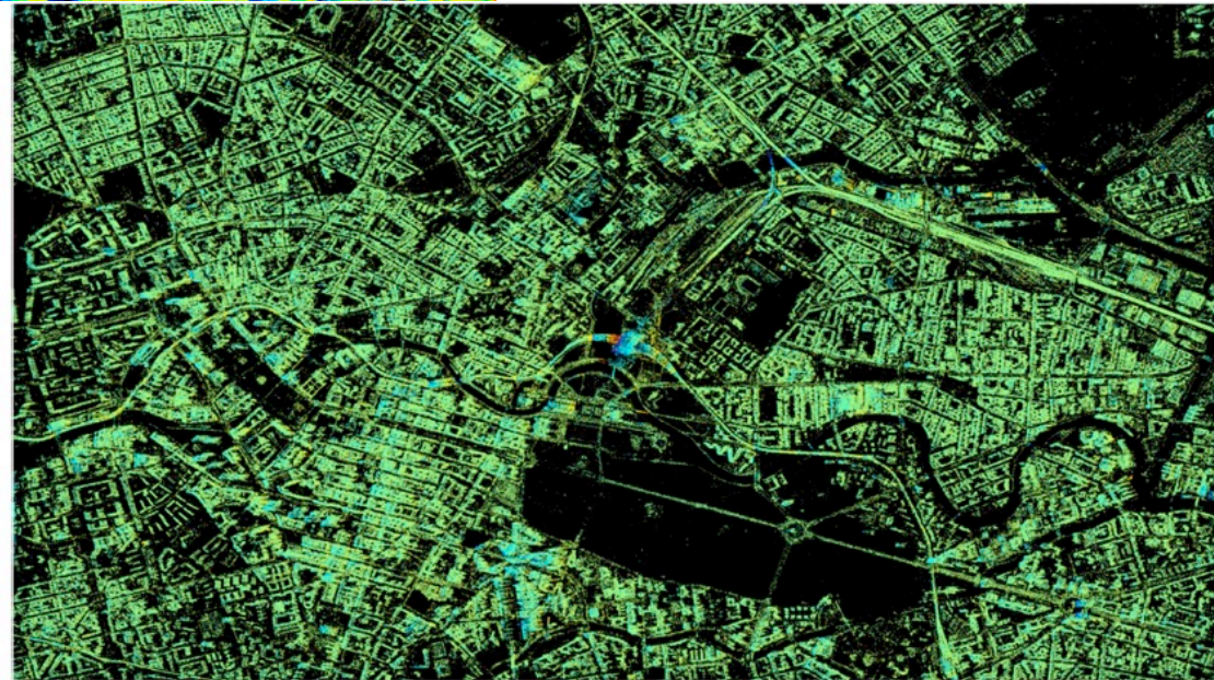
from Zhu et al, 2016 – 3D absolute positioned TomoSAR point cloud from Berlin
