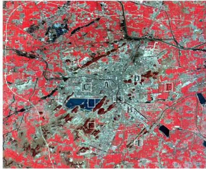
The False Color Image of the Study Area (CBERS 02B-R:Band4, G:Band3, B:Band 2)
