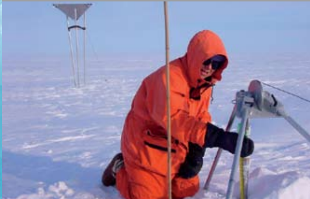
A neutron probe is lowered into a hole drilled in the ice. It collects essential data on snow and ice density layering to help understand the observed radar altimeter signal and ultimately transform the height measurements into net change in ice mass, the main goal of CryoSat over land ice. (Norwegian Polar Institute)
