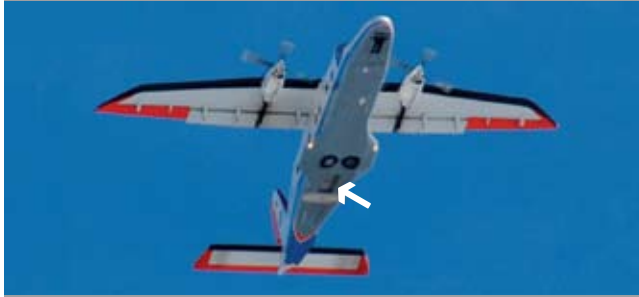
A Dornier-228 aircraft from the Alfred Wegner Institute carrying the 'ASIRAS' airborne version of CryoSat-2's radar altimeter. The rectangular antenna is visible under the fuselage. It provides, together with a laser scanner, the basic measurements required for CryoSat-2 validation. (ESA/M. Davidson)
