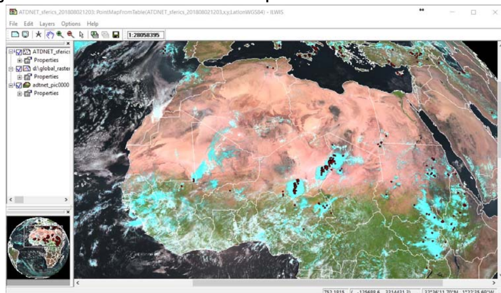
Figure 3.12: ATDNET 15 minutes BUFR file plotted over MSG for the same time step
