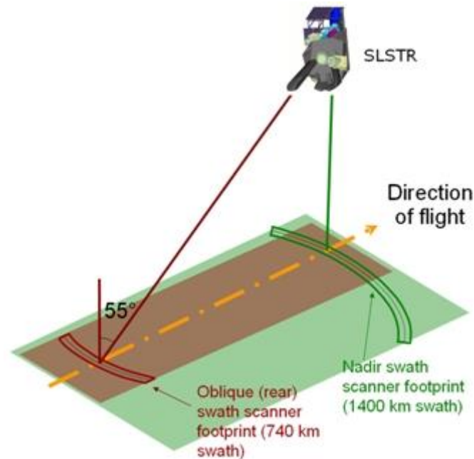
Figure 4-11: Outline sketch of the SENTINEL-3 SLSTR instrument viewing geometry highlighting the asymmetric nadir swath with respect to the nadir point
