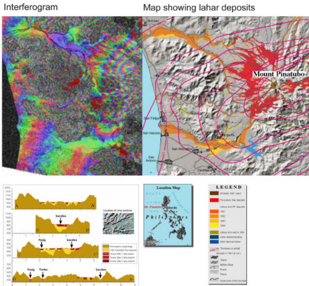
Figure 6 : Left: Interferogram of Mount Pinatubo generated using a tandem pair of ERS images, Right: map showing main deposits related to the 1991 eruption (ash fall, pyroclastic flows) as well as the extension of lahar deposits in subsequent years (partly after: Daag and van Westen, 1996).
