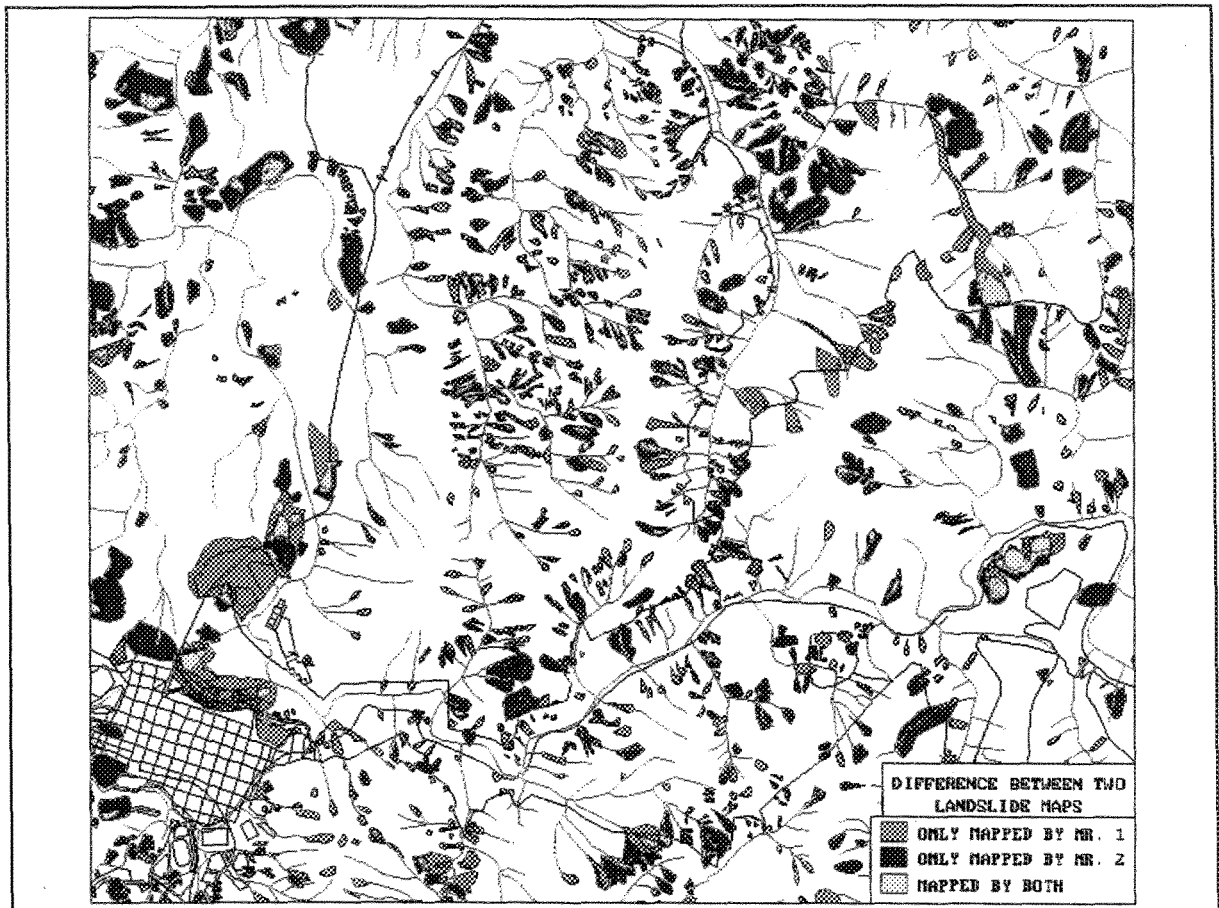
Figure 7.4: Overlay of two landslide maps for a part of the medium-scale study area.
