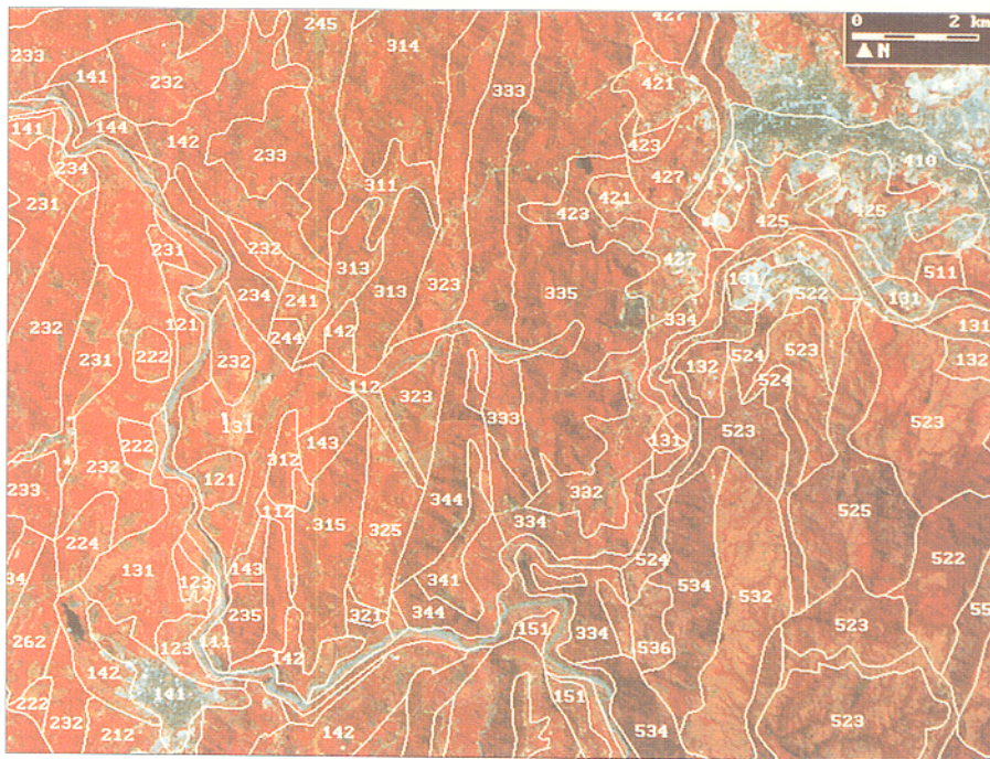
FIGURE 2 Delineation of terrain mapping units obtained by interpreting stereo Spot images of the Manizales region, Colombia
