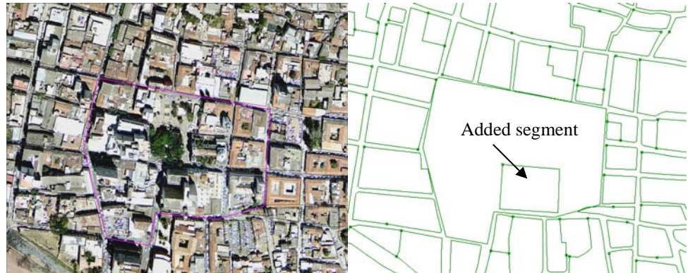
Figure: Left: High-resolution image and right segments of mapping units. One new segment has been added.
