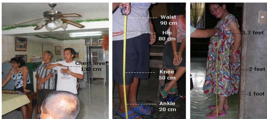
Figure : Measurement of Community-based reference levels for flood depth in centimeters during workshops
