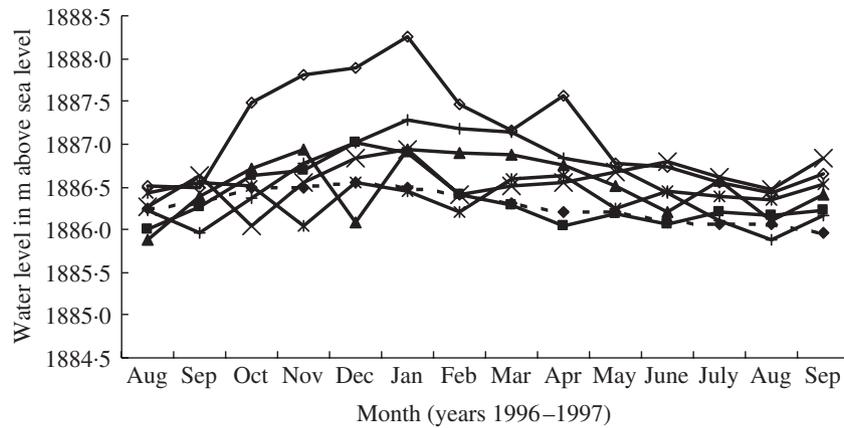
Fig. 1. Observed and forecast water levels at Lake Naivasha for 14 months (1996–1997): ◆, observed; ■, model NN1; ▲, model NN2; ✱, model NN3; ✱, model NN4; ◆, model NN5; +, model NN6
