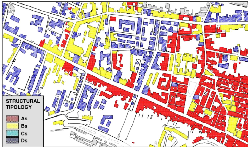
Fig. 3. Torre Annunziata: detail of the vulnerability building classes: A s , B s , C s , D s (EMS-98).
