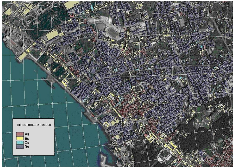
Fig. 15. A detail of the grid with seismic class distribution of the buildings.
