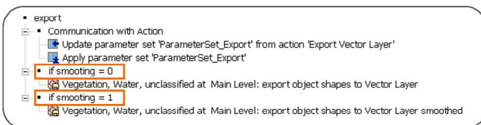
Figure 79: Processes for Action 'Export Vector Layer, using Variable 'smoothing' as condition for execution.
