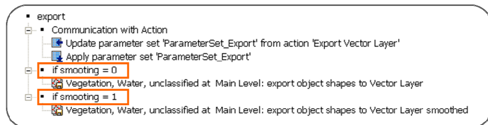
Figure 74: Processes for Action 'Export Vector Layer, using Variable 'smoothing' as condition for execution.
