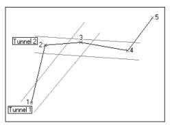
Fig. 1: Tunneling: The first tunnel is constructed around node 1, and intermediate coordinates 2 and 3. Intermediate coordinate 2 falls outside the tunnel and thus remains. The second tunnel is constructed around intermediate coordinates 2, 3, and 4. Intermediate coordinate 3 falls inside the tunnel and is thus omitted. Now that point 3 is omitted, the next tunnel will be constructed around intermediate coordinates 4, 5, and 6 (point 6 is not in this picture).
