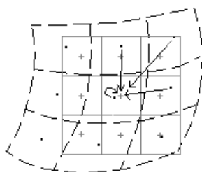
Fig 2: Bilinear resampling. Input pixels are represented by dashed black lines, coordinates of input pixels by black dots; output pixels are represented by solid gray, coordinates of output pixels by gray plus signs. The arrows indicate how output values are determined.
