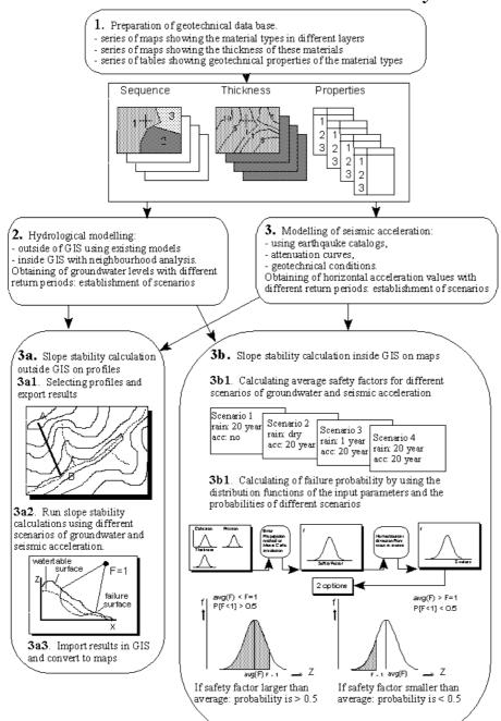
Figure 6.1: Flowchart for deterministic landslide hazard analysis
