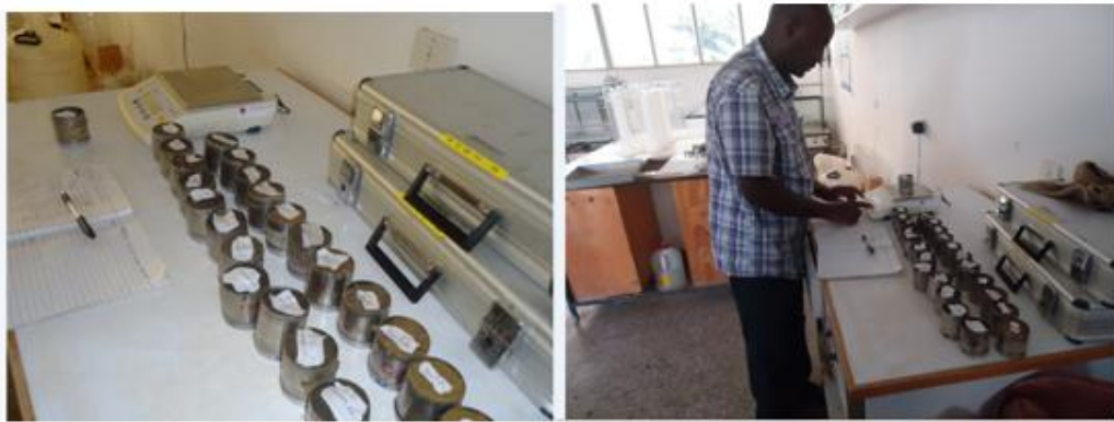
Figure 4-6: Laboratory soil moisture measurement Soil sample collected from the site by core sampler was dried using in the oven dry in Mekelle University and soil moisture were calculated using the following formula.
