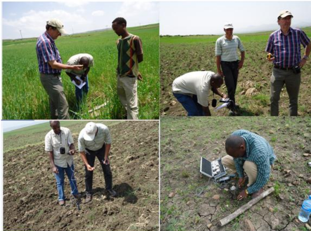
Figure 4-5: Fieldwork soil moisture measurements using theta probe and gravimetric method Adi-gudom, Tigray, Ethiopia. September 14, 2011 to 21, 2011.
