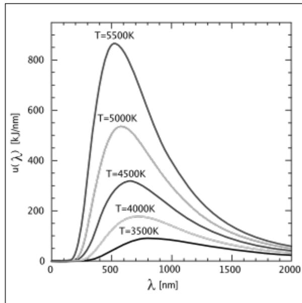
Figure 2. The blackbody curve at 3500, 4000, 4500, 5000 and 5500k
